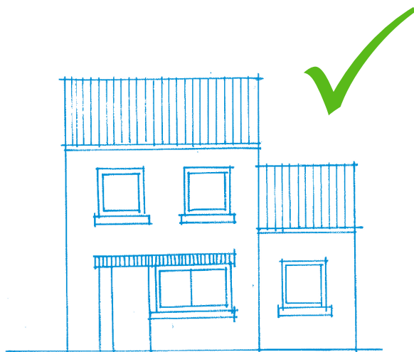
Figure 4.83: Side extension subservient to original dwelling with sympathetic window detail
