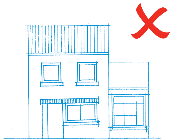
Figure 4.84: Side extension with unsympathetic window detail
