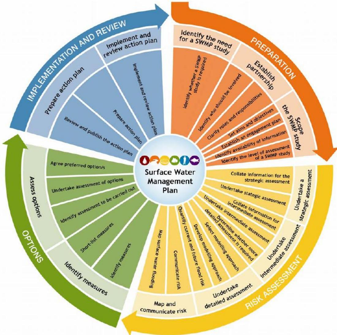
Figure 1-1 Recommended Defra SWMP Process (Source Defra 2010)
