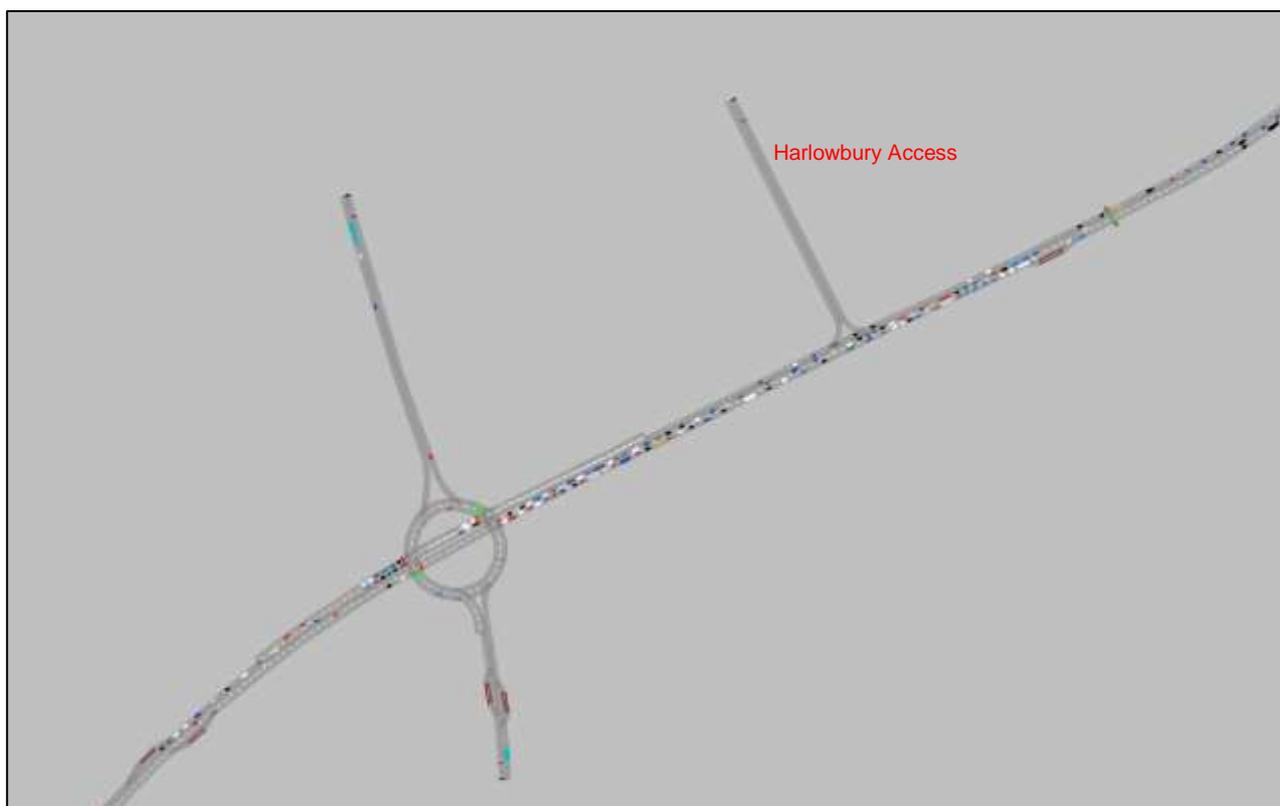
The model of the Emerging Option as shown in Figure 2-7 indicates that this queue would be likely to extend further east past the new access at the East Harlow development (Loading Point 2), preventing traffic from the development from joining Gildea Way at that point. The operation of the Churchgate roundabout was therefore investigated in more detail, as reported in the next chapter, which was primarily a review of the proposed signal timings.
