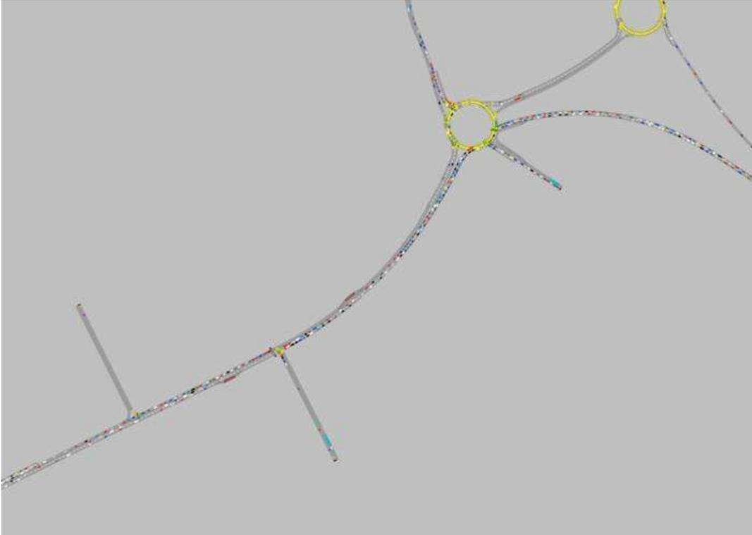
The junction operated slightly better if Gilden Way is widened to two lanes eastbound. However, any benefit was undermined by the fact that the westbound approach would be likely to be oversaturated with queues building up at Loading Point 3 and Sheering Road roundabout in both the AM and PM peaks. The PM peak situation is shown in Figure 3.7.
