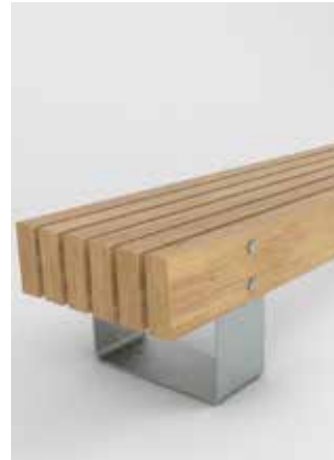
Quay Bench Factory Furniture 3000mm x 530mm x 450mm Slats: FSC® hardwood Frame Hot dipped galvanised mild steel
