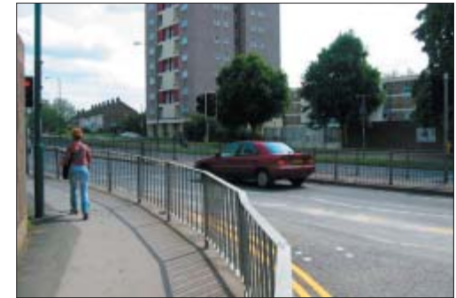
Over control of streets with unattractive street furniture - rails restrict desire lines and fail to cater for pedestrians
