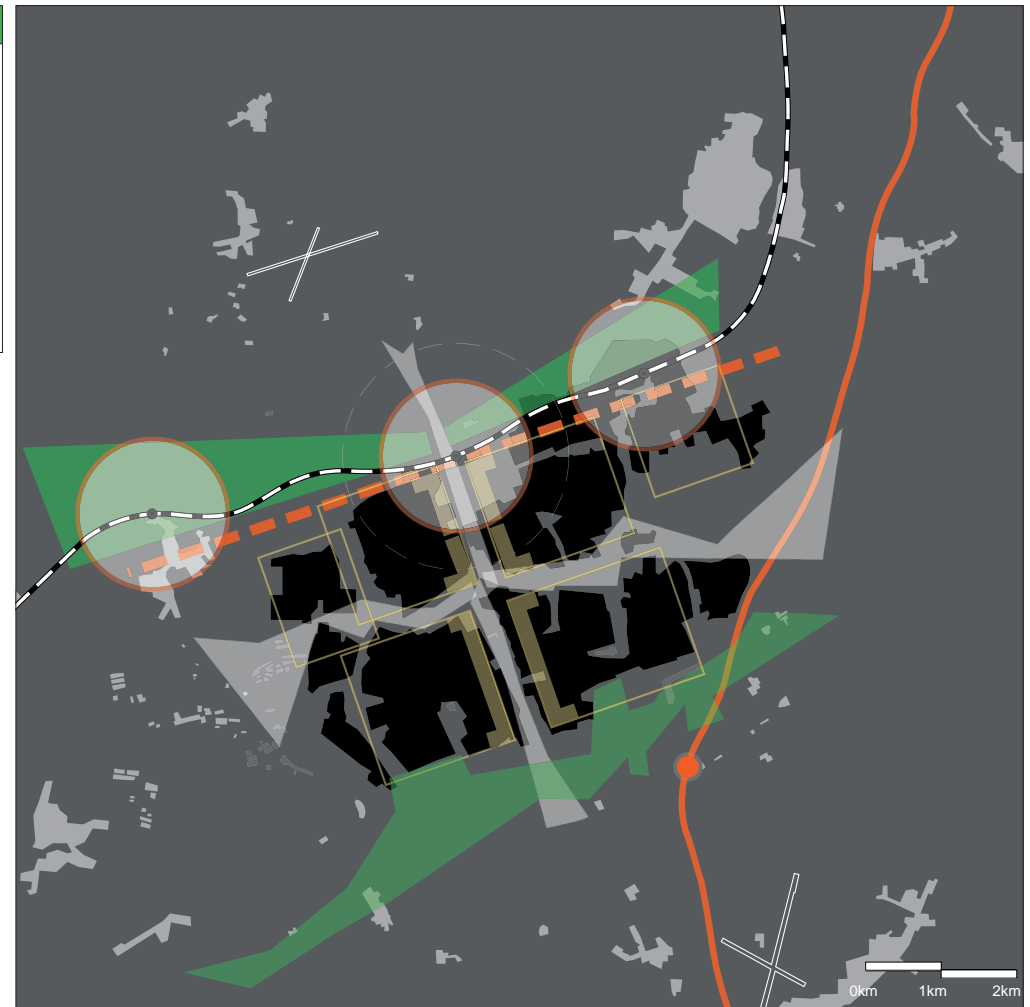
Figure 5.3: An improved public transport system with higher ridership would achieve principles of reducing resource consumption in transport. Harlow's generous open space network provides the opportunity to retrofit a new high quality Public Transport system supporting higher density development along possible future alignments.
