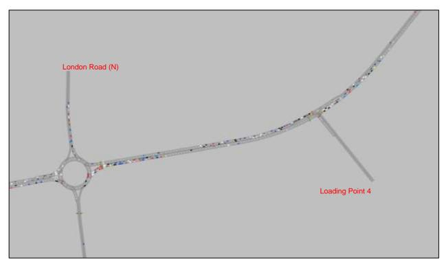
The proposed junction design would be expected to result in reduced queueing on Gilden Way eastbound and on London Road southbound. As shown in Figure 3-3, a small queue remains on Gilden Way eastbound in the PM peak, however this no longer be likely to extend to the London Road roundabout. The queues from the development at loading point 4 would also be likely to be reduced in the AM peak as a result of the junction redesign.
