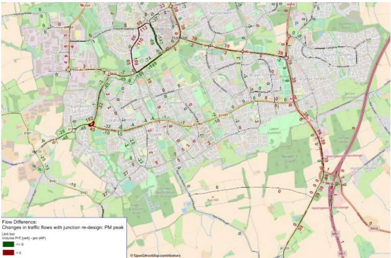
Figure 5-16 - Changes in Wider Harlow Development Traffic Flow with Junction Re-Design – PM Peak Hour
