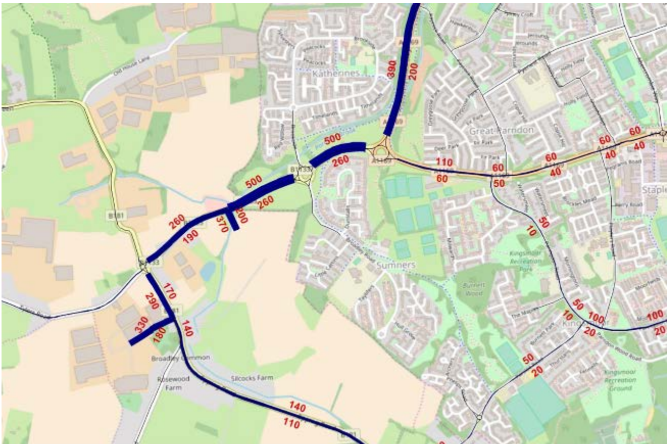
Figure 4-3 – Detailed View of Traffic Assignment from and to West Katherine's and West Summers
