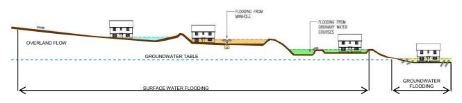
Figure 1-8 Illustration of Flood Sources<sup>1</sup>
