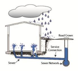
Figure 3-9 Surcharging of the sewer system (left) and internally within a property (right)
