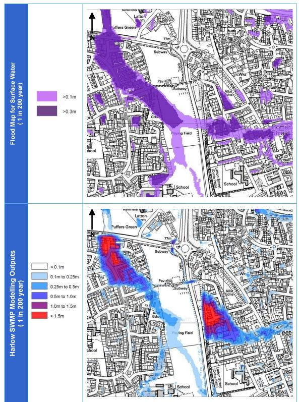
Figure 3-6 Example comparison between FMfSW and SWMP model outputs
