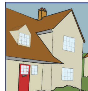
An example of a gable fronted roof extension
