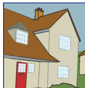
An example of a hipped roof extension
