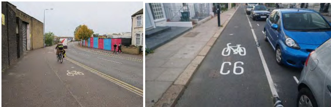
Figure 6-9: Blackhorse Lane (left) has installed narrow cycle tracks alongside the existing footway with a small kerb upstand, and Cycleway 6 (right) has used light segregation to provide cycle tracks in narrower sections of the route
