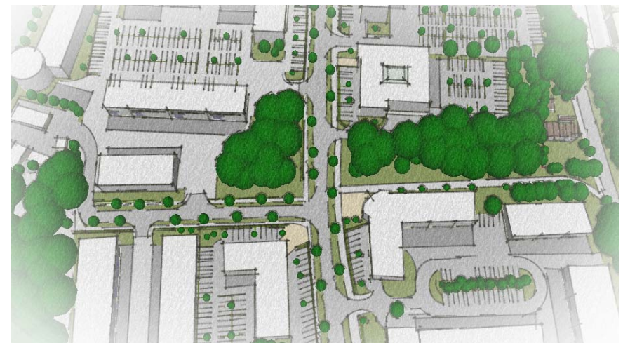
Public right of way upgraded along the central corridor of the site to form a new landscaped entrance for walking and cycling and an important access road to fringe sites towards the western boundary of the site and electricity substation.
