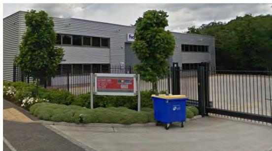
Above, gates set back by 6m from the carriageway to ensure long vehicles can gain entrance to sites without obstructing the highway.
